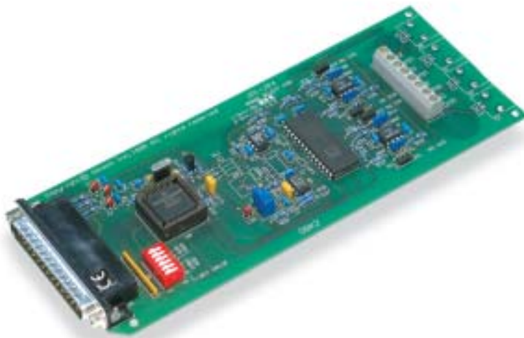
The 4-channel DBK2 allows systems to generate precise bipolar analog voltage outputs
